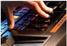
Part Balance sliders The Part Balance sliders let you quickly adjust the volumes of each of the four parts.
